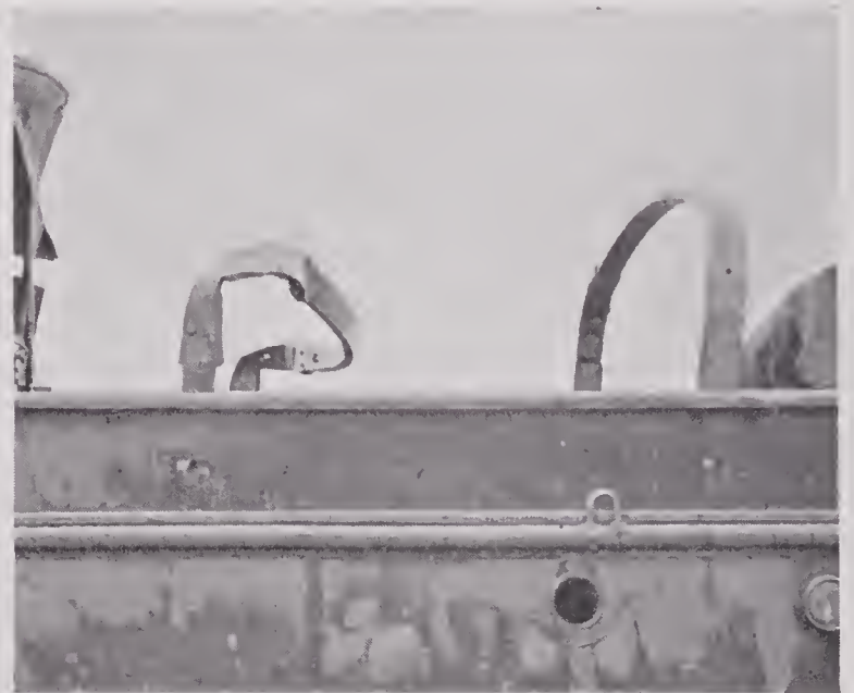
FIGURE 37. Steel-jointed wooden cargo bows deformed by surf impact.
